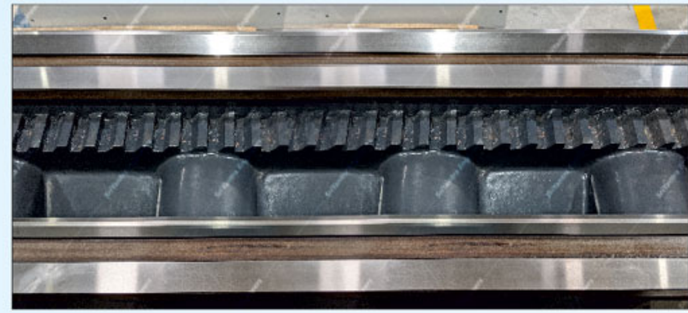
Heavily Ribbed Bed with Generous Bed width proportions
