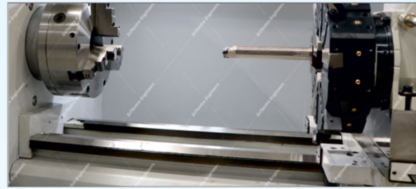
Longitudinal Bedways: Induction Hardened to 400 – 450 BHN and Precision Ground
